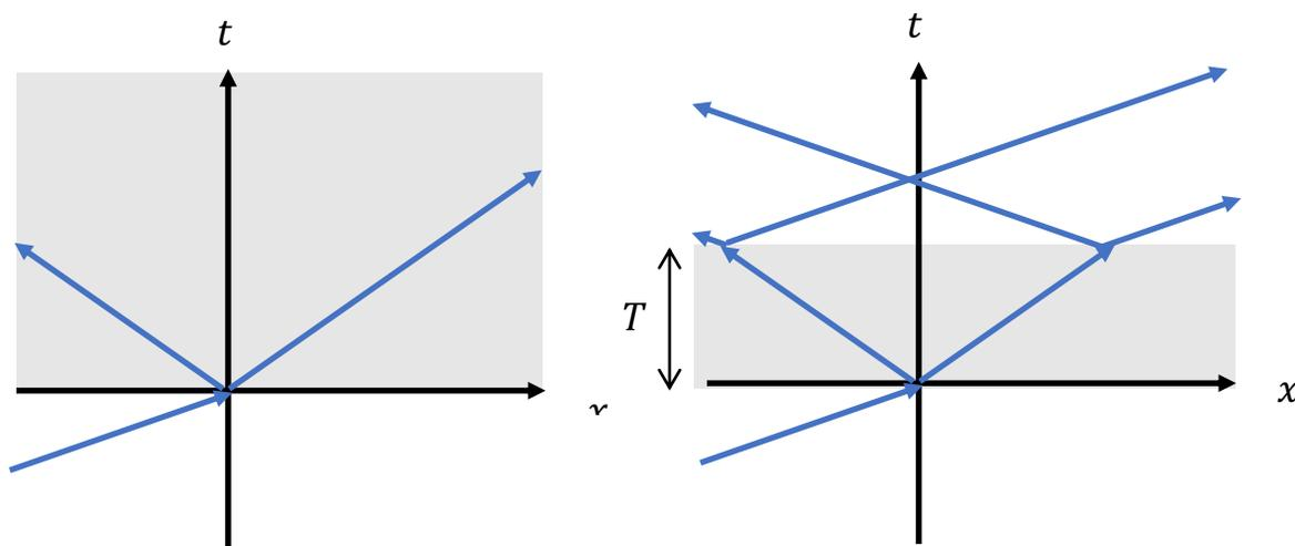
Fig. 2: (Left) Schematic diagram for a light ray entering a time-boundary in which the permittivity changes from  $\epsilon_1$  to  $\epsilon_2$  (Right) Schematic diagram for a light ray going through two time-boundaries. The permittivity changes from  $\epsilon_1$  to  $\epsilon_2$  at  $t = 0$  and changes back to  $\epsilon_1$  at  $t = T$ .
