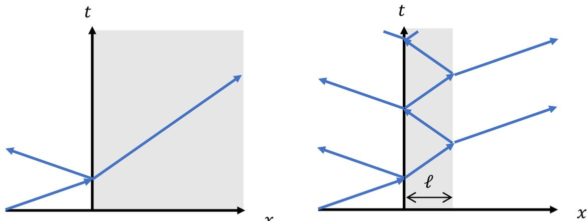
Fig. 1: (Left) Schematic diagram for a light ray entering an interface between vacuum and dielectric medium (Right) Schematic diagram for a light ray entering a slab of dielectric medium undergoing multiple reflections.
