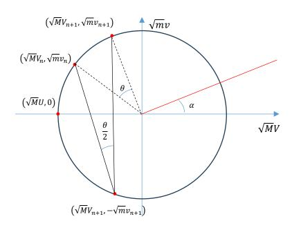
It can be seen that for consecutive collisions between the two blocks, the angular position increases by  $\theta$ , and is  $n\theta$  just before the  $n^{th}$  collision. Hence
